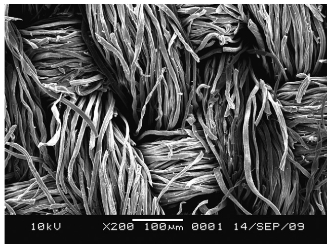
Fig. 4. SEM photograph of degraded residue of nano-cellulose hybrids in nitrogen.
